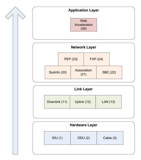
In addition to each Component/Process state code, the terminal maintains a *System State Code* that indicates the overall state code for the terminal. Typically this is the *lowest* process state code as the system state code works as a layered model (similar to OSI Network Model).
